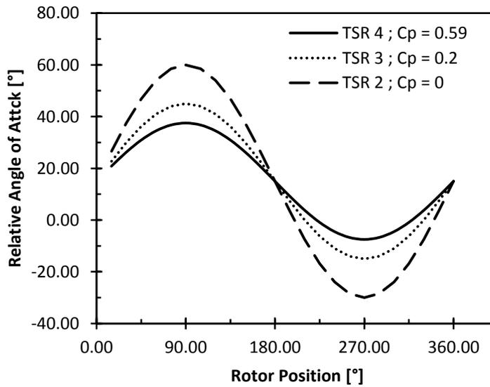
Figure 6: Transient angle of attack at various tip-speed-ratios at all rotor positions
