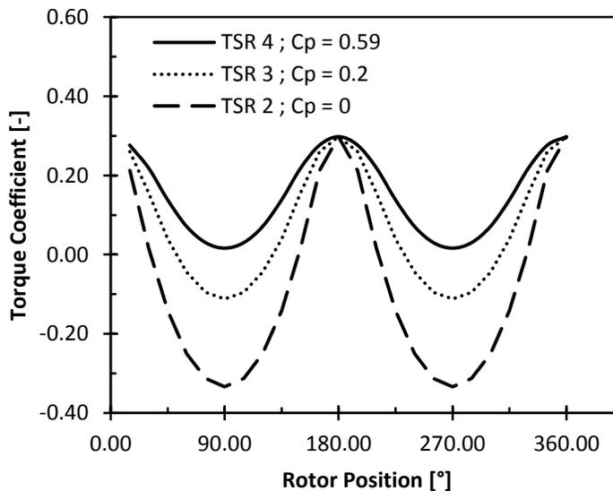
Figure 7: Torque coefficient of various tip-speed-ratios at all rotor positions
