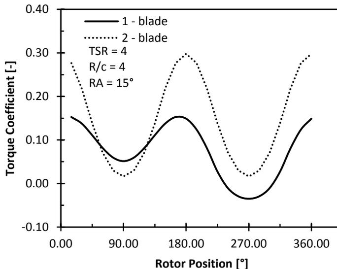
Figure 3: Predicted Torque on a VAWT at all angular position of rotor rotation
