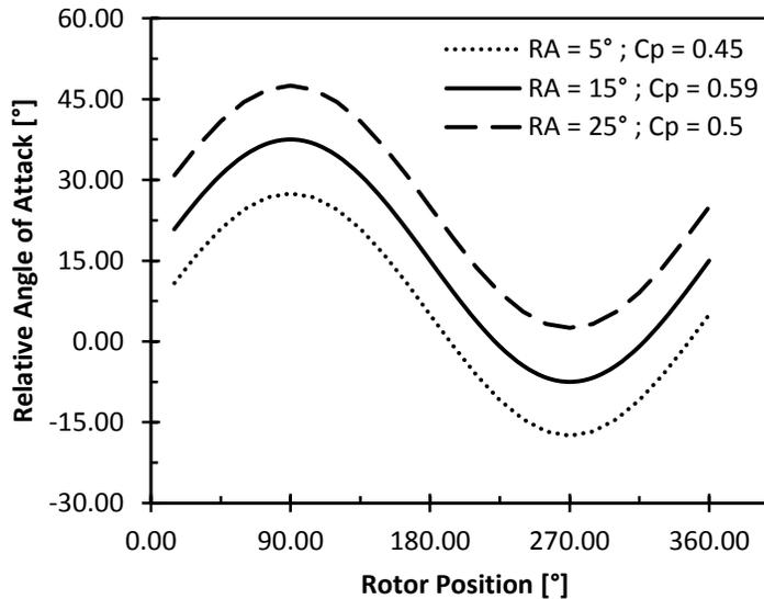
Figure 9: Transient angle of attack at various rigging angles at all rotor positions
