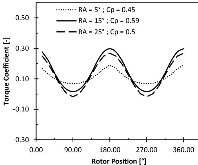
Figure 8: Torque coefficient of various rigging angles at all rotor positions
