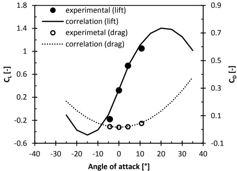
Figure 2: Lift and drag performance of a Clark-Y (B) airfoil
