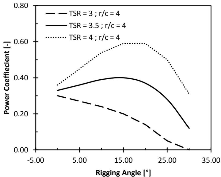
Figure 5: Predicted performance of a VAWT with various tip-speed-ratios
