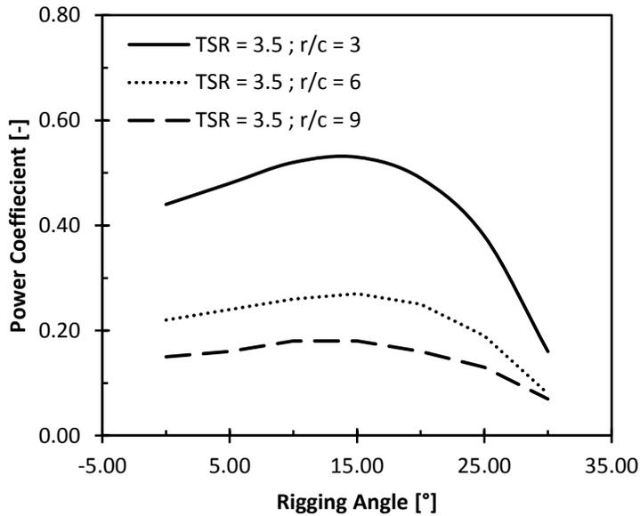
Figure 4: Predicted performance of a VAWT with various blockage ratios
