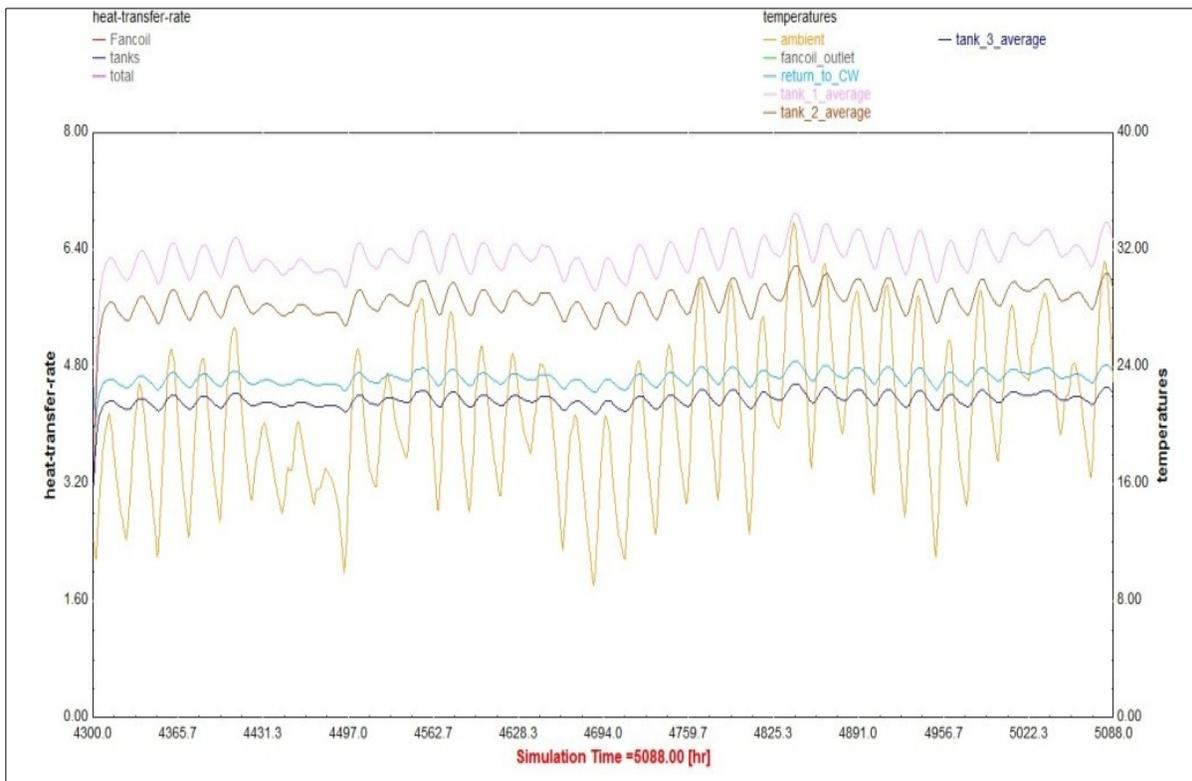
Figure 7: Simulated tank temperatures
