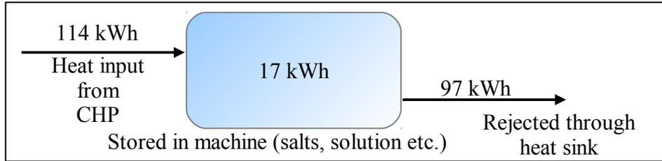
Figure 2: TCA Energy transfer when charging (Double mode) [11,14]
