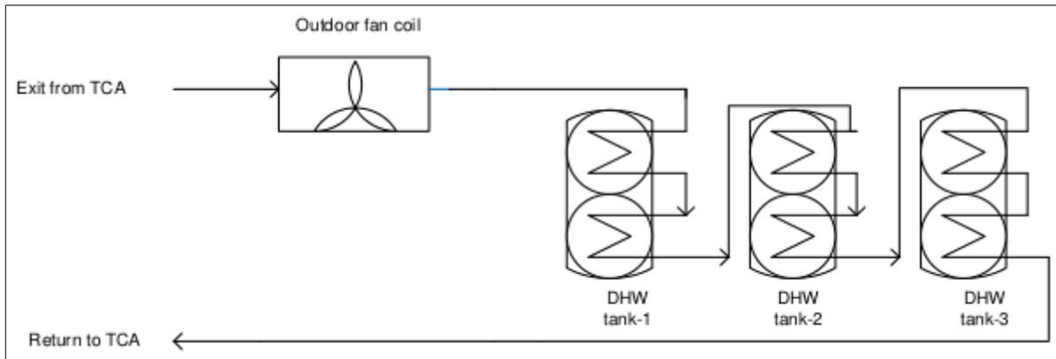
Figure 6: Simulated heat rejection circuit
