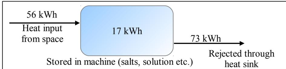
Figure 3: TCA energy transfer when discharging (Double mode) [11,14]
