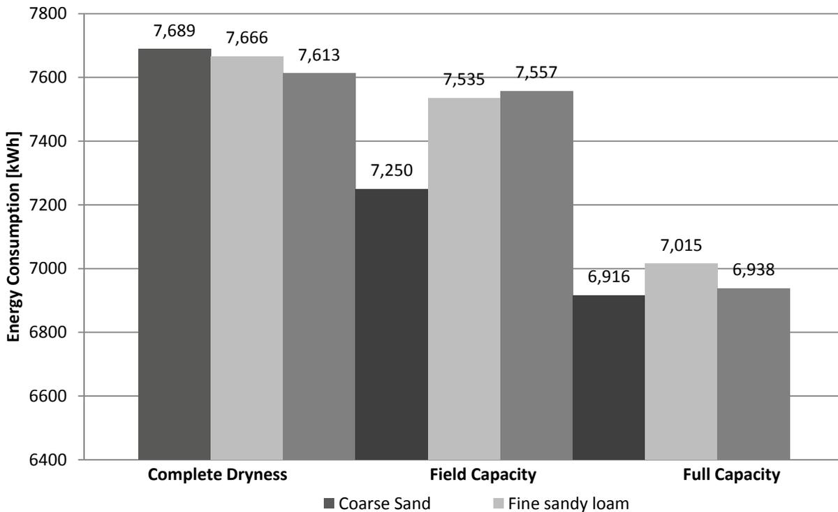
Figure 7. Variation in heat pump electricity consumption at three different water contents for all three soil types under investigation.
