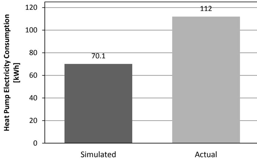
Figure 5. Comparison between actual and simulated heat pump electricity consumption for the cooling period from August 23<sup>rd</sup> to September 14<sup>th</sup>, 2010.
