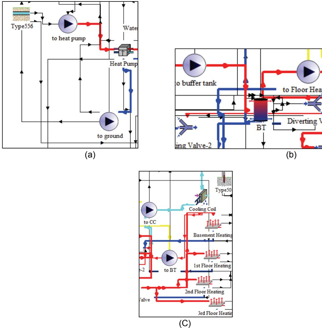
Figure 4. Three major sections of the HVAC system as modeled in TRNSYS. a) Heat pump-to-ground, b) Heat pump-to-buffer tank, and c) Buffer tank-to-AHU/in-floor heating.
