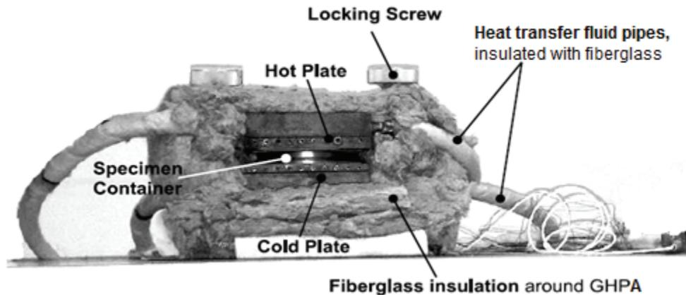
Figure 1. Guarded hot plate apparatus (GHPA) used to measure soil thermal conductivity [2].
