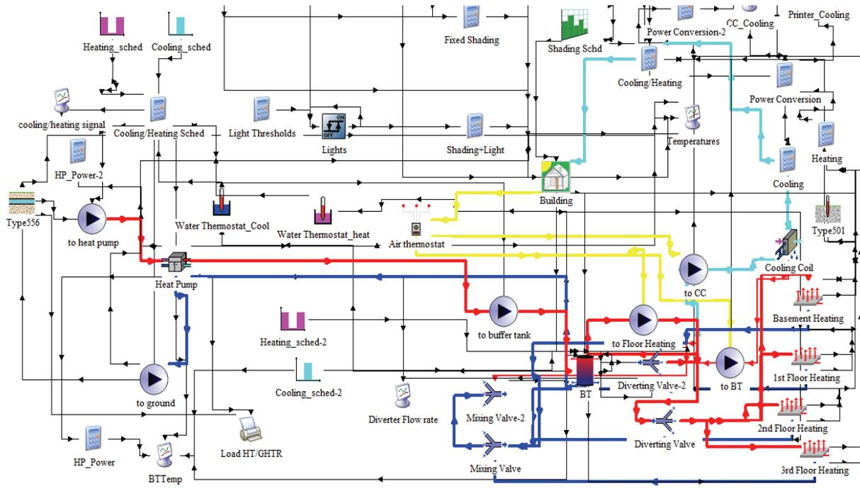
Figure 3. An overview of the TRNSYS model of the HVAC system.
