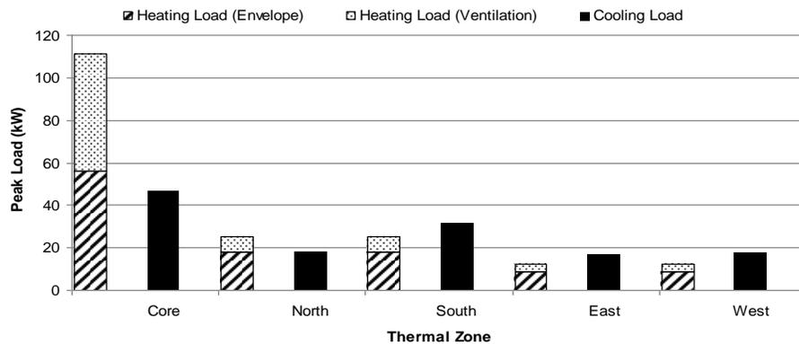
Figure 4. Peak thermal loads for large office
