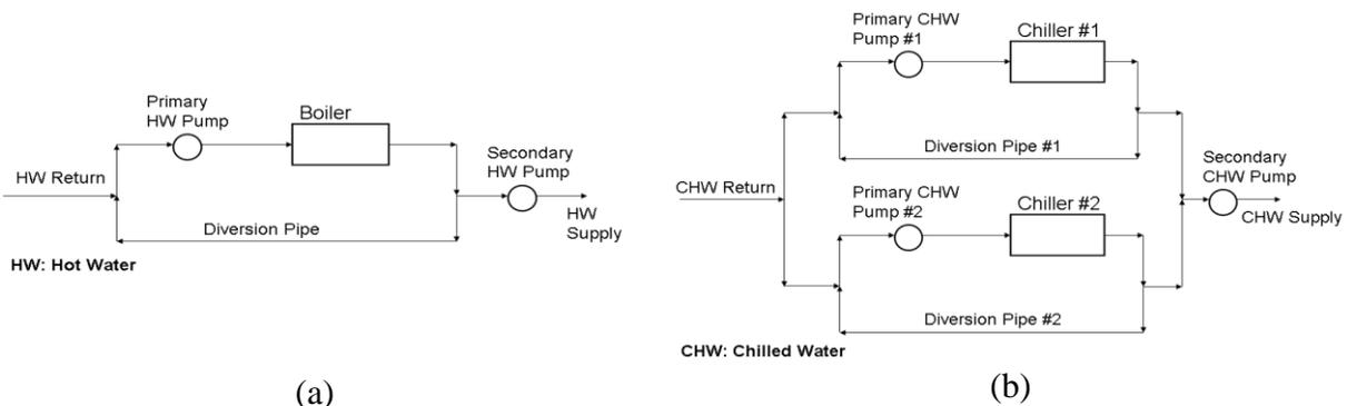
Figure 2(a). Heating system for large office
