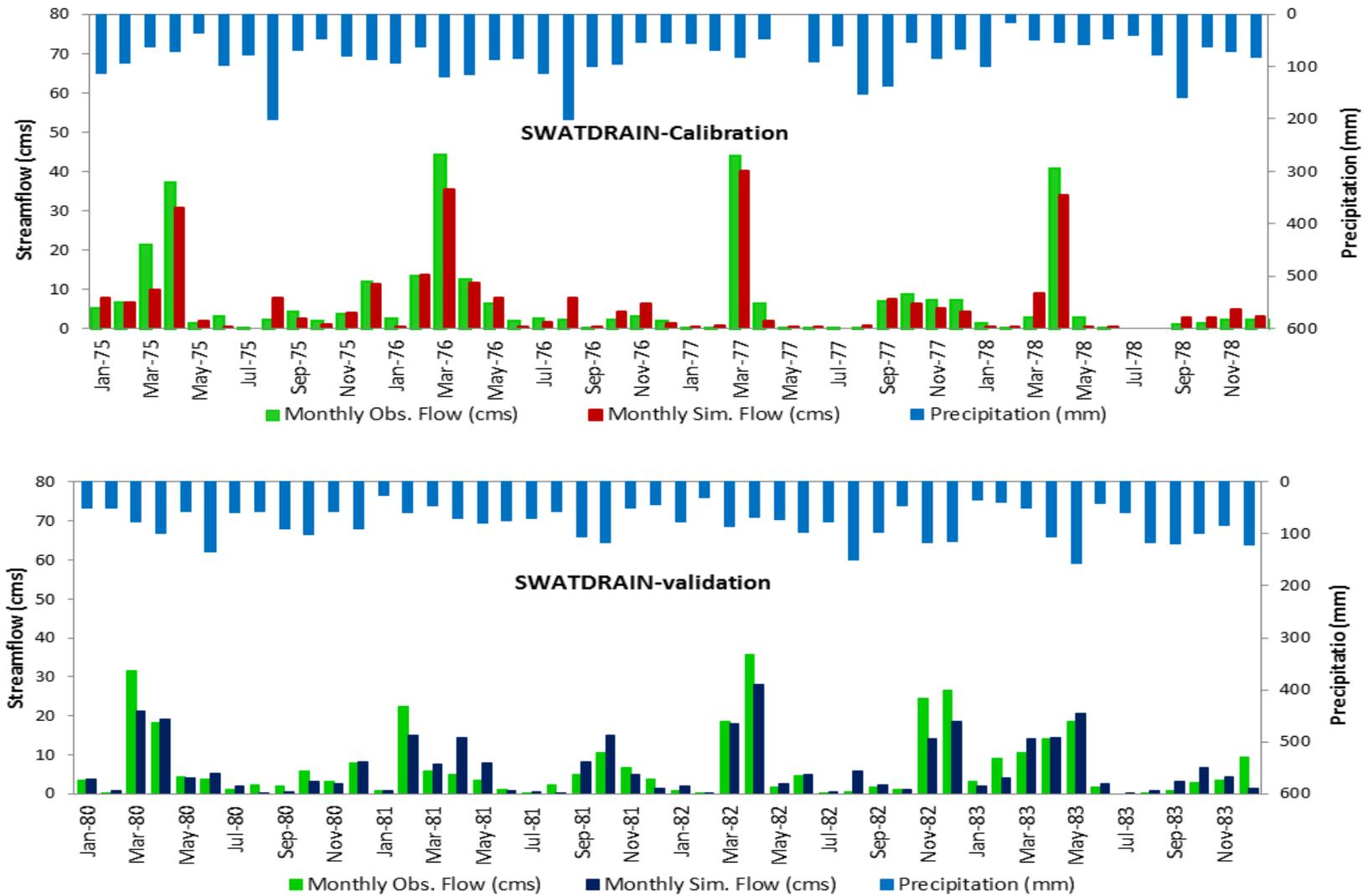
Figure 2. Monthly streamflow for Canagagigue watershed during calibration and validation period
