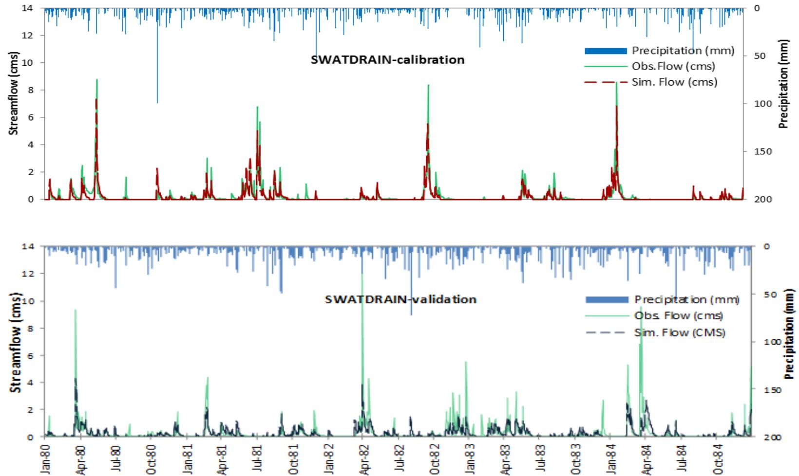
Figure 3. Daily streamflow for Canagagigue watershed during calibration and validation period
