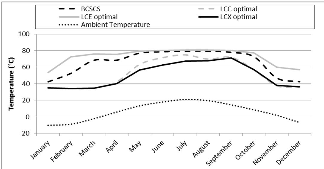
Figure 6. Average monthly tank temperatures in the domestic hot water tank
