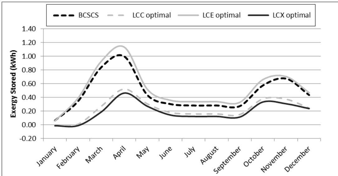
Figure 7. Monthly exergy storage profiles of the radiant floor tank
