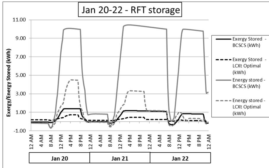
Figure 3. Exergy and energy storage profiles for the radiant floor tank for January 20-22
