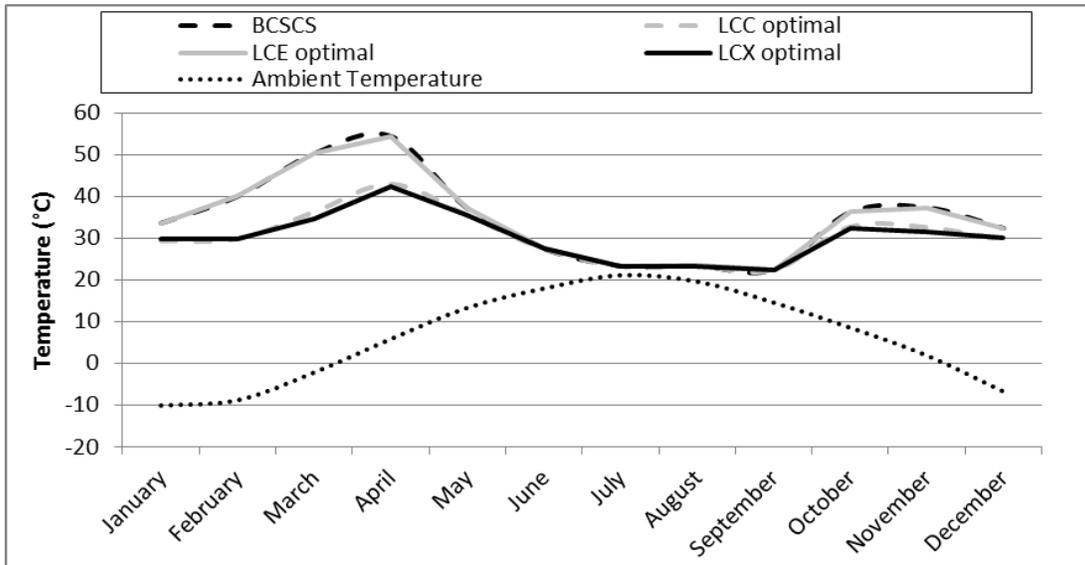
Figure 5. Average monthly tank temperatures in the radiant floor tank
