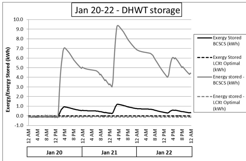
Figure 4. Exergy and energy storage profiles for the domestic hot water tank for January 20-22
