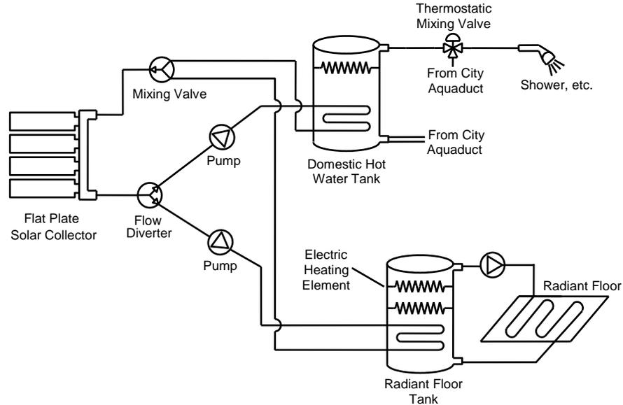
Figure 1. Schematic diagram of the solar combisystem [8]
