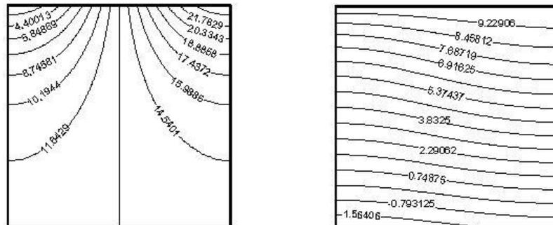
Figure 3. Distribution of the head (left) and temperature in the case  $W=0, R=0, K=0.1$ .
