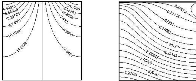
Figure 4. Distribution of the head (left) and temperature in the case  $W=0, R=0, K=0.5$
