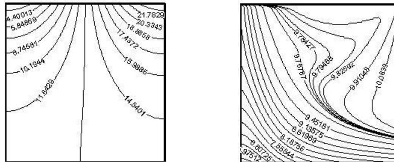
Figure 5. Distribution of the head (left) and temperature in the case  $R=0.01, W=0.1, K=0.5, D=0.064$
