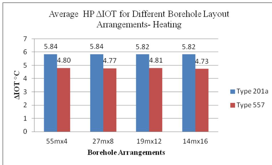
Figure 7- Average heat pump differential IN and OUT fluid temperature (HP  $\Delta IOT$ ) for different borehole layout arrangements in heating mode.
