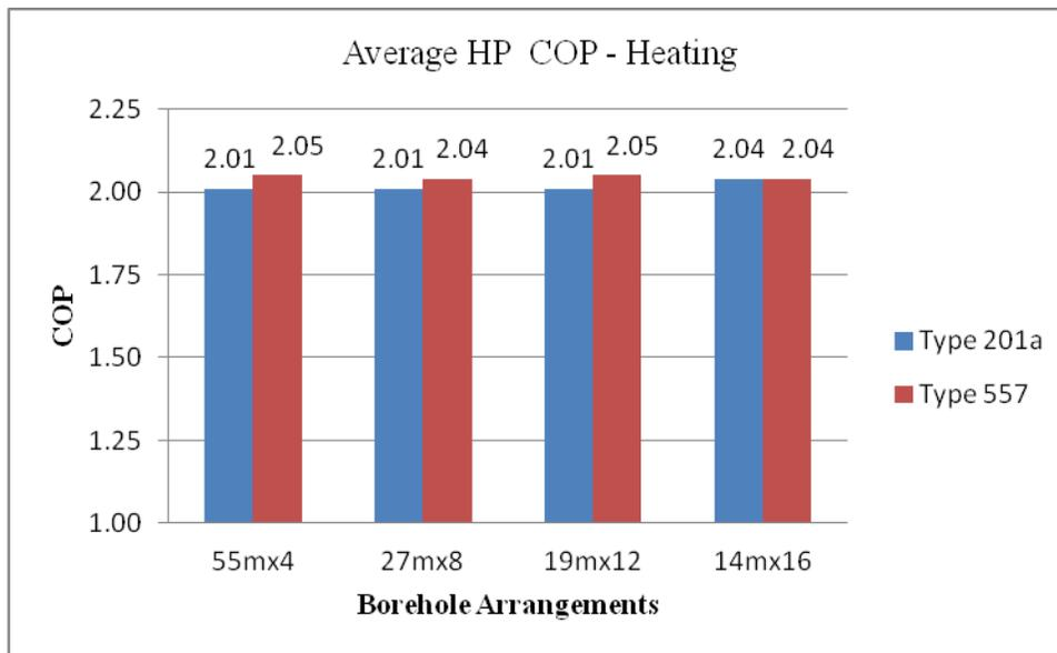
Figure 9- Average heat pump Coefficient of Performances (COPs) for different borehole layout arrangements in heating mode.
