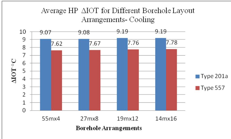
Figure 8- Average heat pump differential IN and OUT fluid temperature (HP  $\Delta$ IOT) for different borehole layout arrangements in cooling mode.
