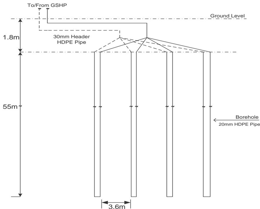
Figure 1- Ground loop borehole layout.
