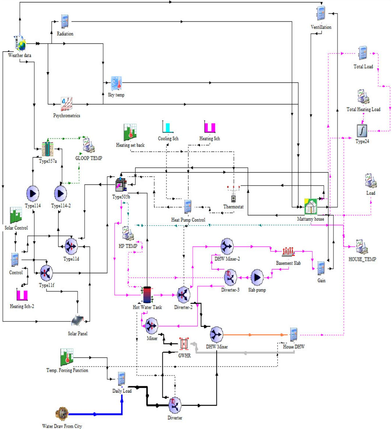
Figure 2- TRNSYS model layout
