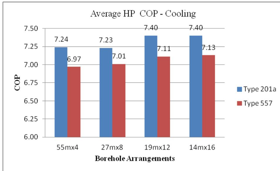
Figure 10- Average heat pump Coefficient of Performances (COPs) for different borehole layout arrangements in cooling mode.
