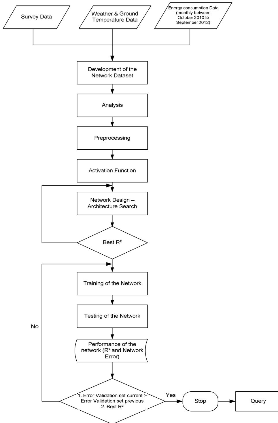
Figure 2: Flowchart depicting the methodology used for the development of the ANN model.
